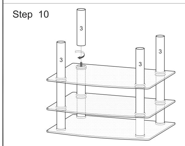
Screw cylinders (3) onto long rods (A). Note that cylinders (3) will fit snuggly inside the decorative rings placed in the previous step.
